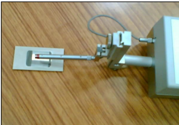
Fig 10: Calibrating view with Measuring Instrument (Surtronic 3+)
